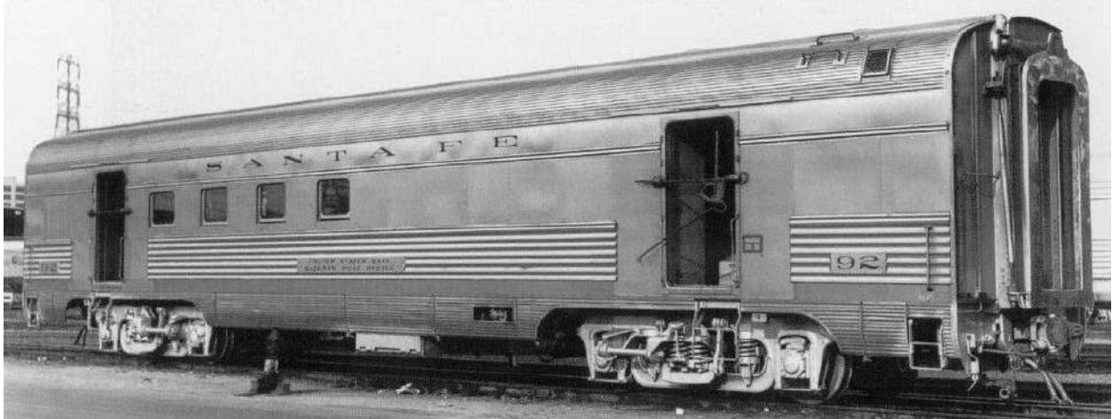
#92 with full skirts and 41CDO-II trucks. Robert Loewing photo, Dennis J. Kogan collection, from Ellington & Shine, Head End Cars .
