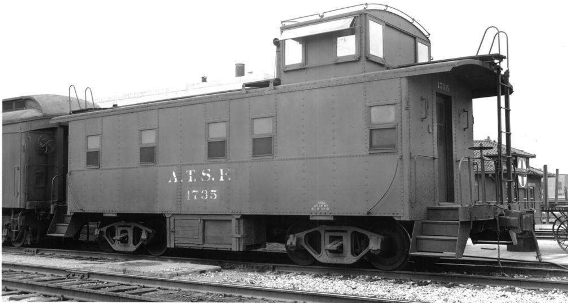
Caboose 1735 repainted but in original condition Repacked AC 9-30-41 Series 1650-1749 ACF built 1928
