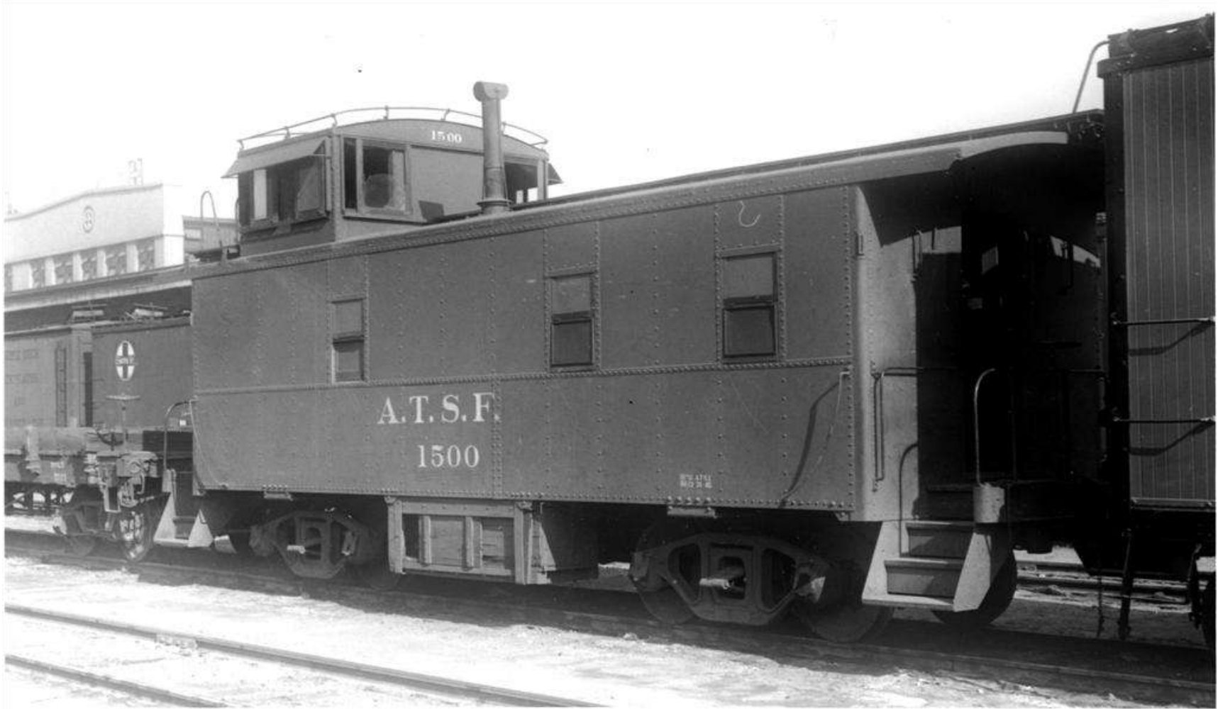
1500 at San Bernardino “J” Side hand grabs replaced with curved Still lettered in the 1938-1944 lettering scheme
