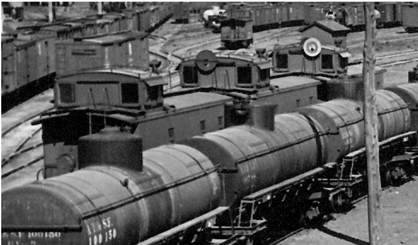
Wig-wags on steel cabooses Style 7 (right pivot) and Style 6 (left pivot)
