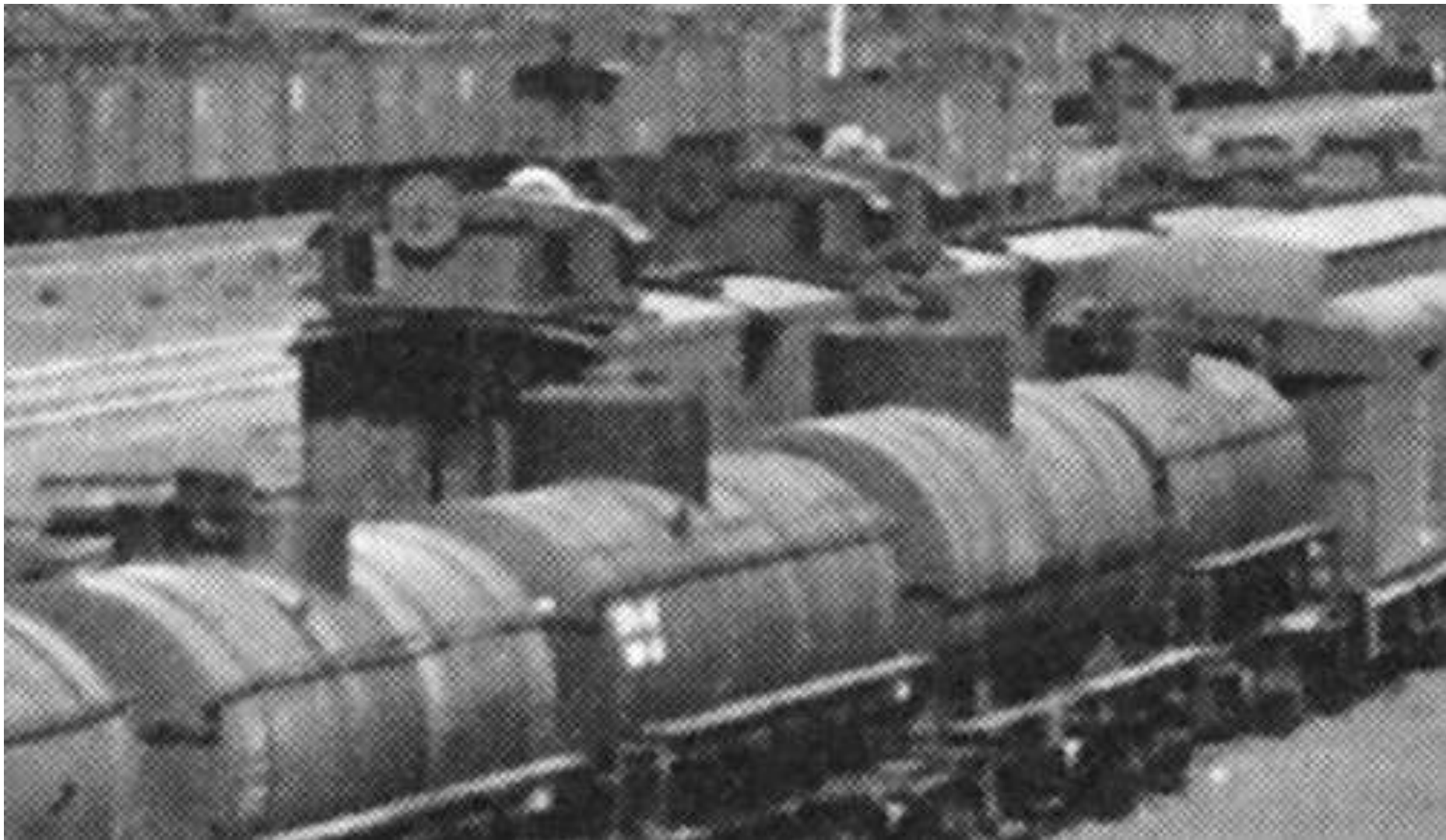
Three steel cabooses with Style 7 wig-wags (right side pivot)
