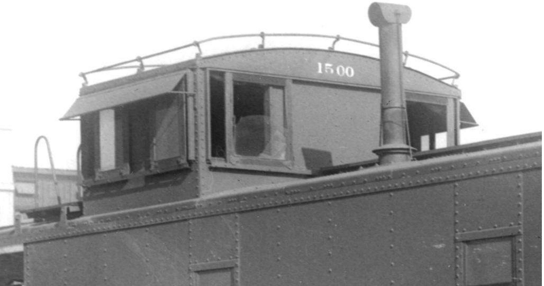
1500 shows changes to the cupola hand grab configuration Note the 5 brackets across the width of cupola
