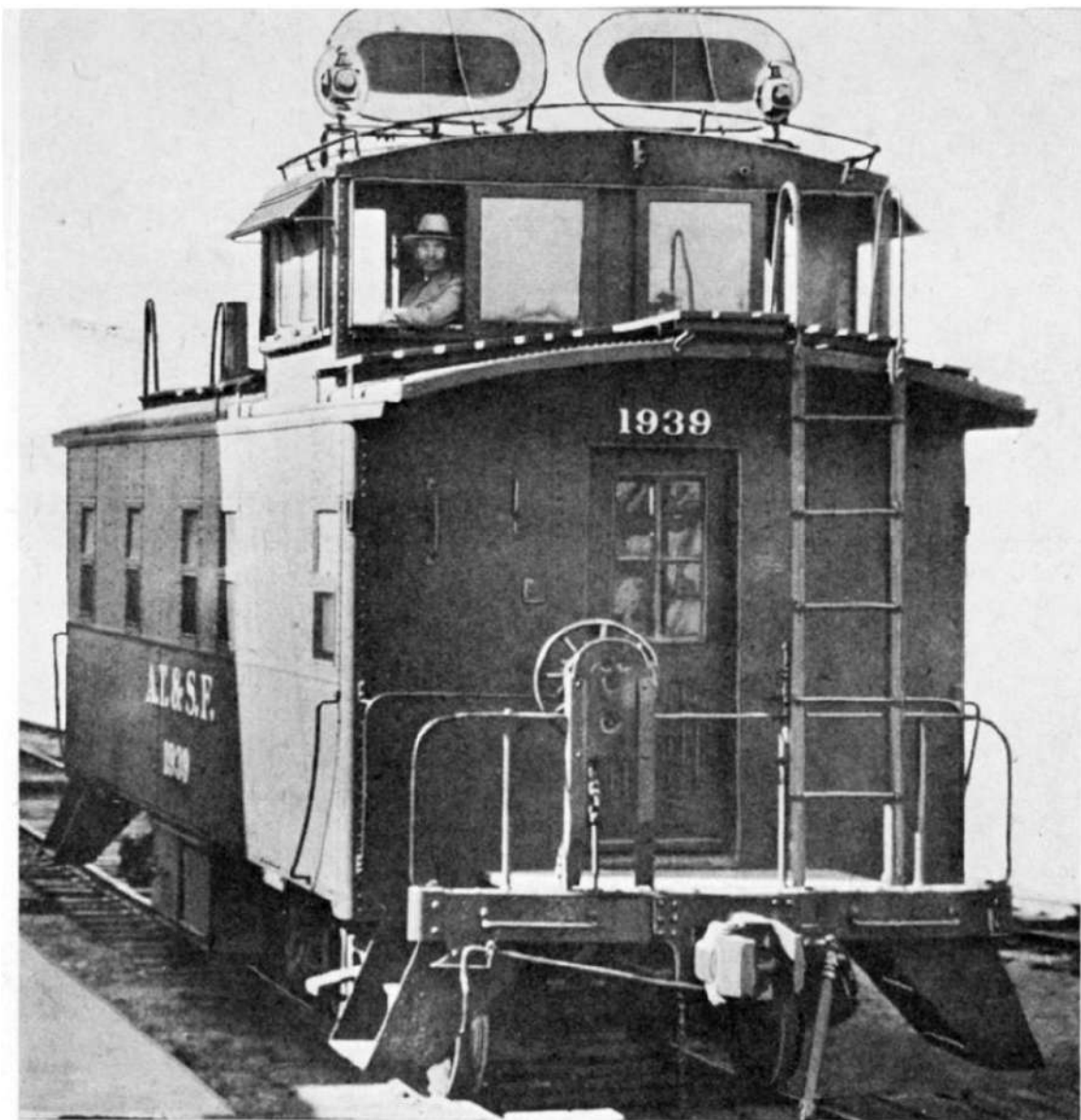
Ever see a way-car equipped with Marcum airbrake signal? Indicators would be in this position, crosswise to car, if a train were coupled ahead and brakes set.
