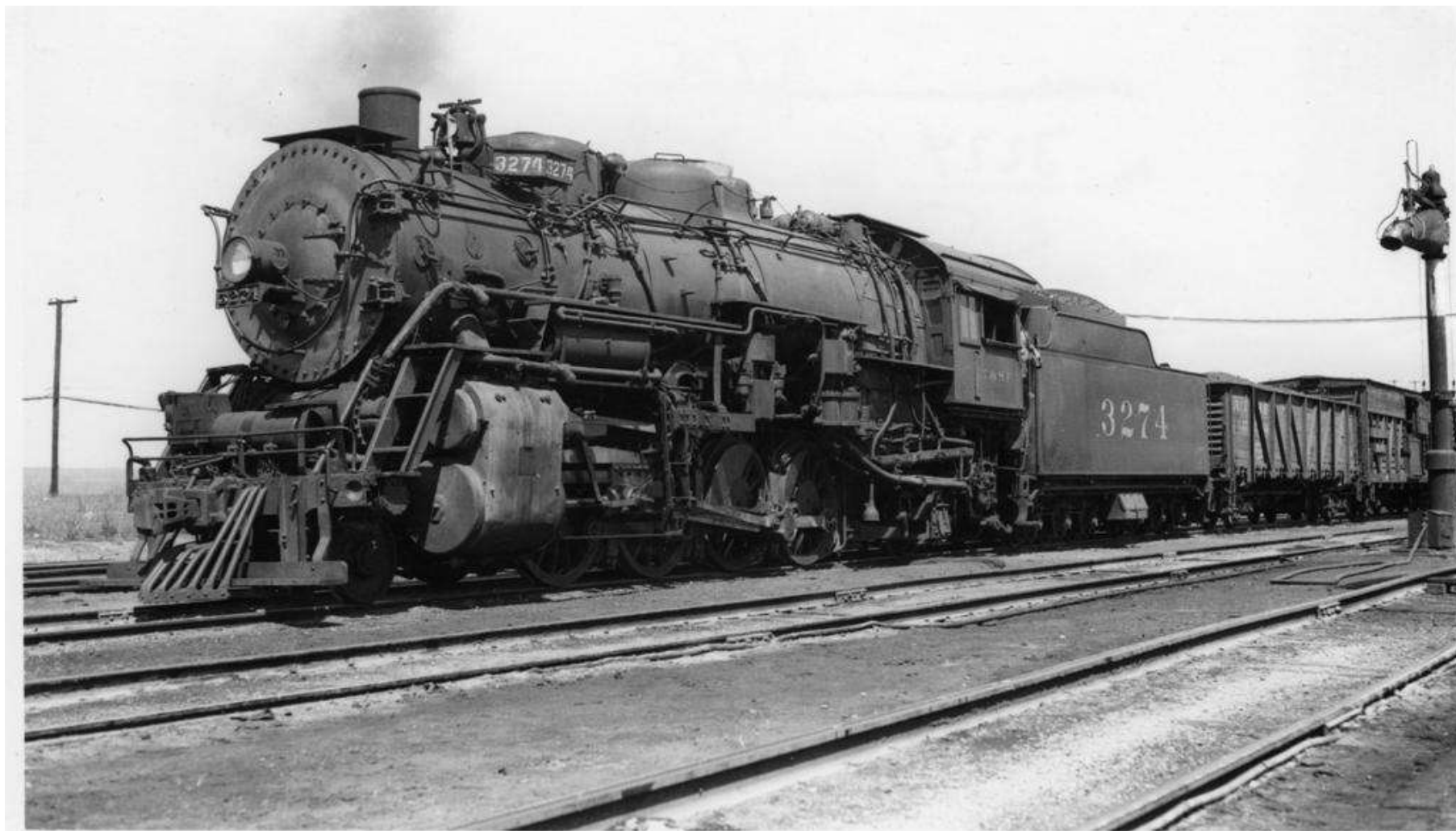
3274 Chillicothe 1948 radio antenna ground plane in front of stack
