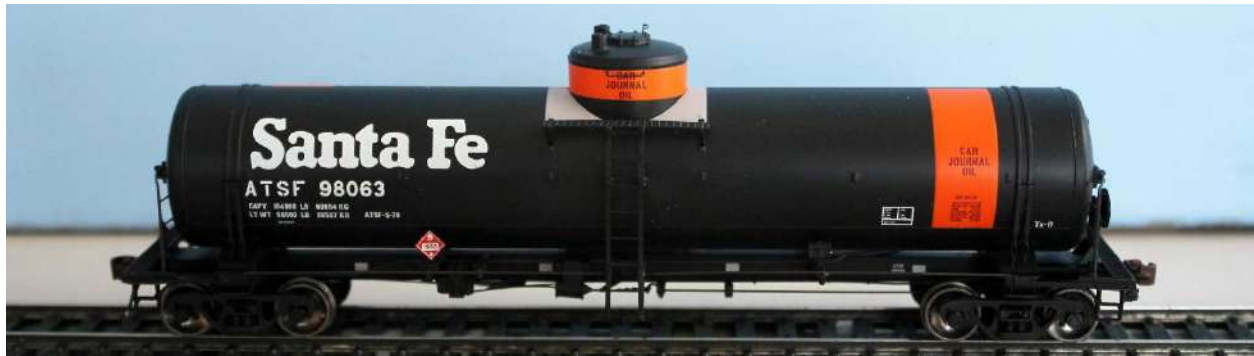
American Limited model of ATSF 98063 (Tk-O as rebuilt in May 1978 for car journal oil service. The paint scheme is post-1982 because of the presence of the simplified consolidated stencil.)
