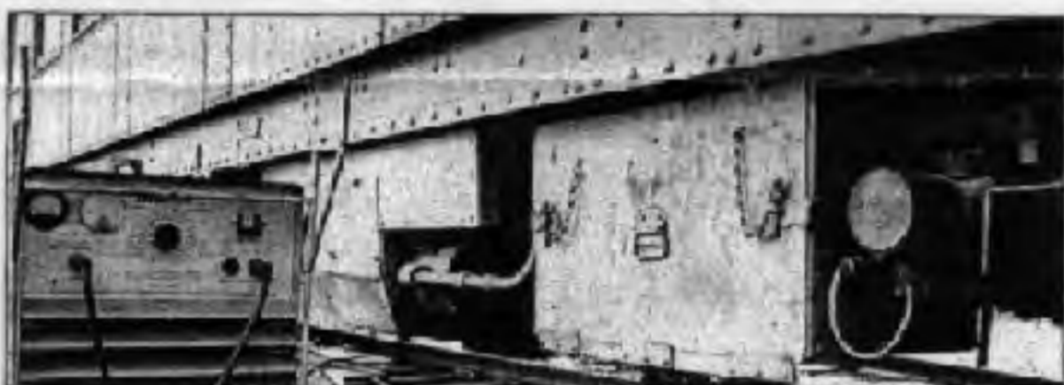
Variation of the valve closet on 3231 is also on the same side of the car as the air duct and the battery box. Box at right was sometimes separated from unit at left on diners and lounges. Arc welder had taken root and could not be moved and obviously is not a part of system!
