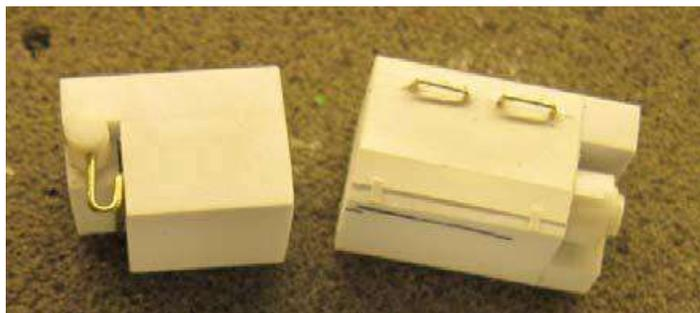
Remove the water tank, battery boxes, single generator and the single A/C box. Re-position the battery boxes and the water tank on the other side of the car. Add the coupler cut levers if desired. The original Chair car underbody is on the top and the modified underbody is below it.
