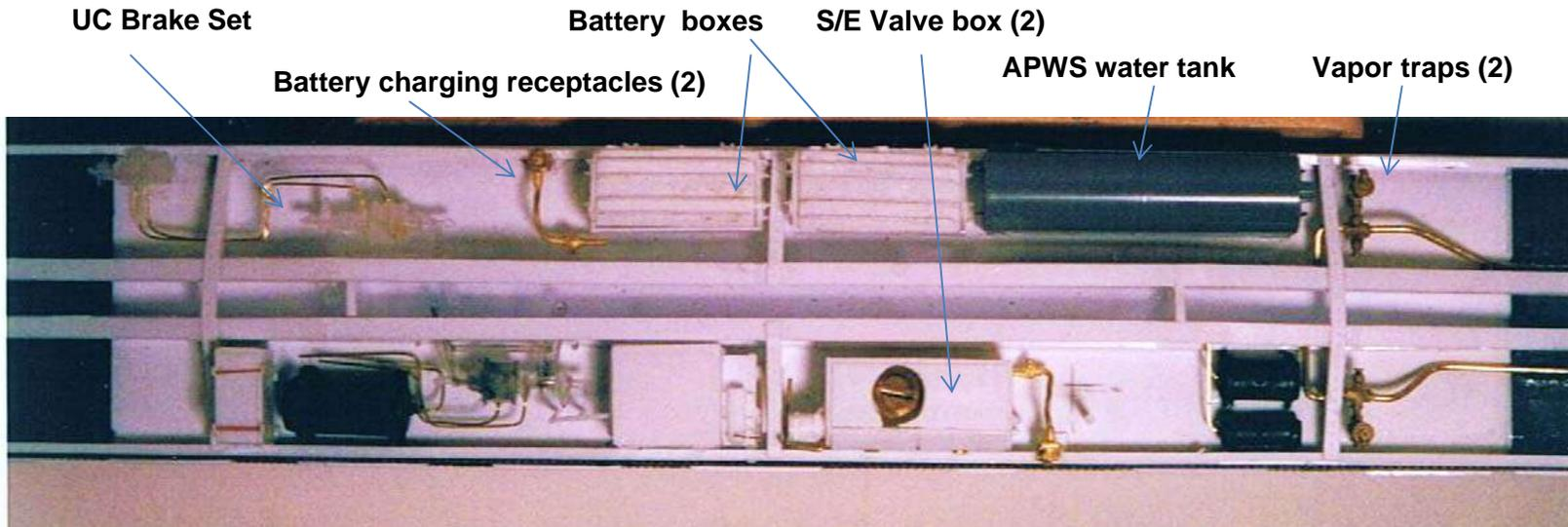
Cut away the flat side channel & replace with true 3D channel: (Evergreen .100")
