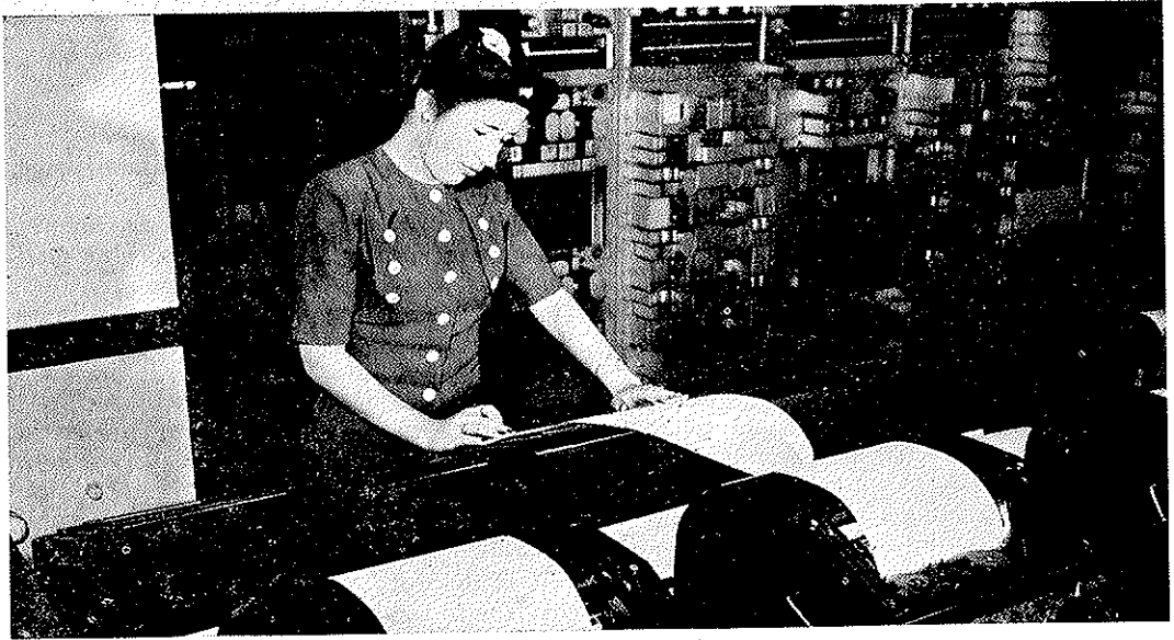
PRINTING-TELEGRAPH machines are located in 96 printer offices throughout the Santa Fe system. Such important items as wheel reports, advance switch lists, and data included in the main line red ball freight reporting system are transmitted. Here is a close-up of a printer in action, receiving.
