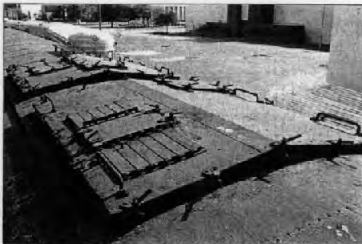
Close-up of hatch detail on parlor-club 3231 at Fair Park in Dallas. The shutters for the air outlet dampers (see Figure 1) are clearly detailed. Object ahead of the a/c unit is an induction radio antenna. This car was converted in 1935 from a parlor/observation.
