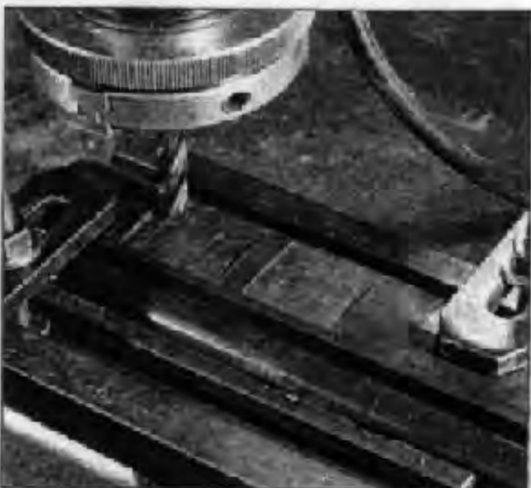
A carbide end-mill on the Unimat is used to mill out the Walthers roofs to accommodate the flat bottomed castings. I cut as far down in the roof as I could. Note the dogs to hold the roof.
