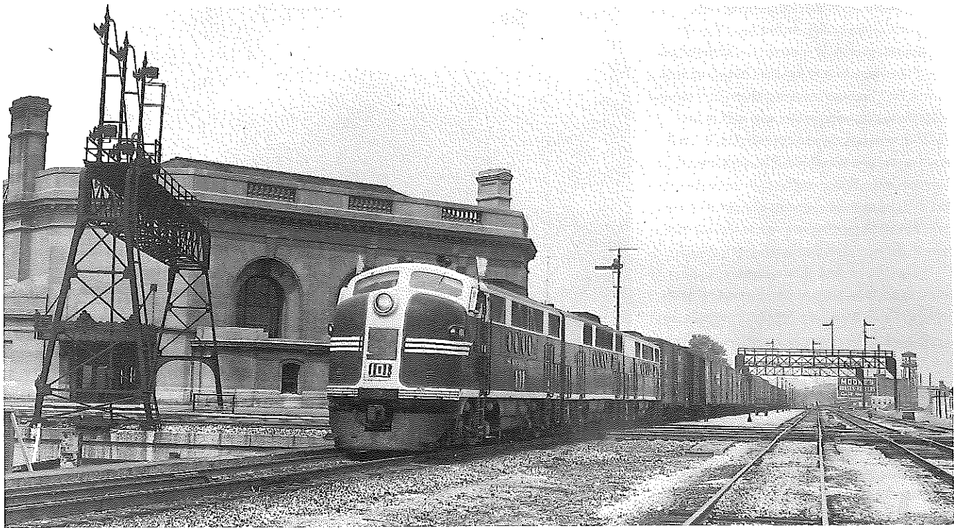
The 101 clumps across the Rock Island at Joliet, above, with a westbound, displaying what no self-respecting FT model should be without: the white flags of an extra. Note that one (or both) of the boosters are running backward, not that it matters. And it appears on close inspection of the photo that the vermilion stripe stops at the cab door. August 2, 1949. -Wally Abbey
