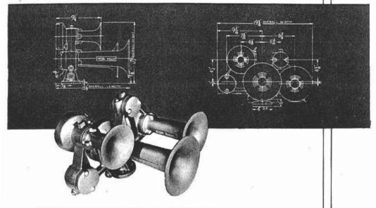
M5-124 The 5-chime base used in the Model M5-124 Nathan Airchime comes fitted with three powerful bell units (1, 2, and 4) base openings 3 and 5 being sealed off with blanking covers. Bells 3 and 5 may be easily added at any time service requirements warrant by removing the covers and replacing with the proper bells. The M5-124 ensures ample warning for standard passenger and fast-freight road use, though volume and fullness of tone do not equal that of the 5-chime complement. Weight 28 pounds.
