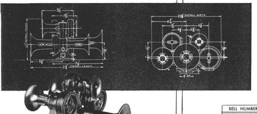
M5R24 This is the same grouping of five Airchimes as in Model M5, except that bells 2 and 4 have been reversed on the base for greater warning coverage to the rear. The tone combinations used achieve a pleasing and highly effective signal of great penetration in both directions. Weighs 35 pounds.
