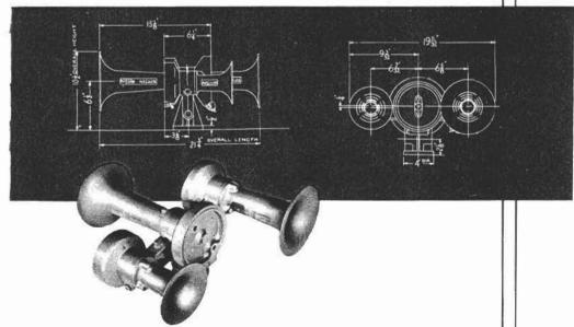
M3R1 This is the same assembly as the M3, but with bell 1 reversed for more signal range to the rear. General tone and range are entirely satisfactory for the type of service for which the unit is intended, and will ensure an extra safety factor for freight and switcher operations. Weight is 28 pounds. Uses bells 1, 2, and 4.
