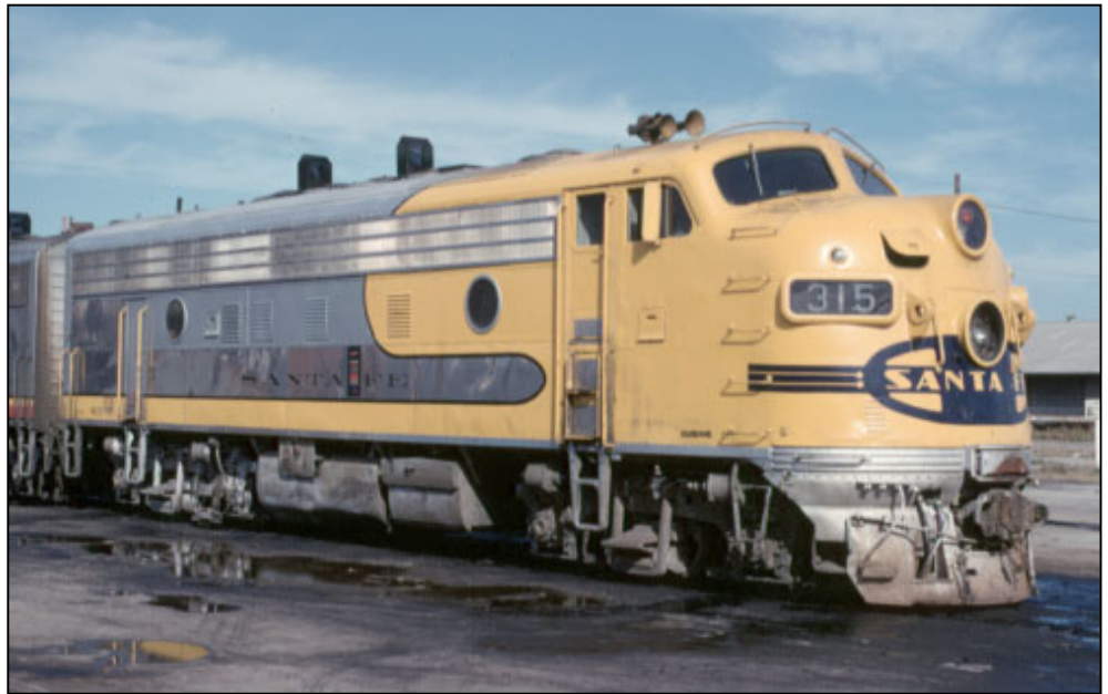
ATSF F7 315L rests at Houston Union Station on December 31, 1972. Note the 'CLEBURNE' maintenance stencil on the front of the unit and the Farr vertical-slit stainless steel side grilles that replaced the horizontal-slit grilles early on. The 315L was a Phase I early F7 and renumbered into the 300 Class as 315L from the 37 Class 40L. —Ralph Back
