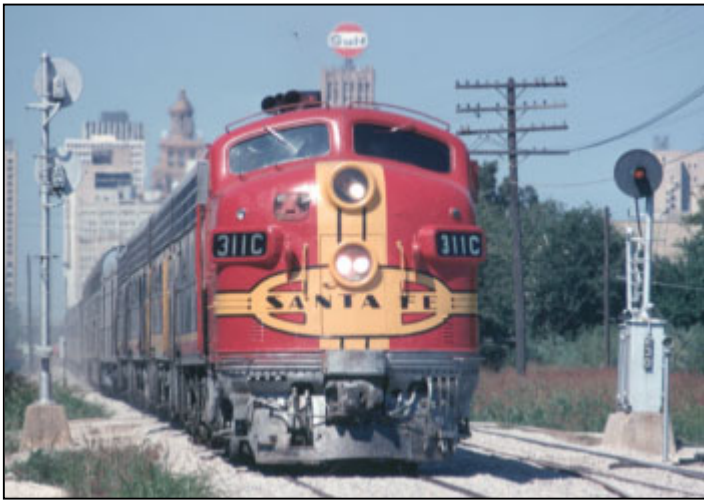
Left: Look closely at the second unit behind F7 311C and you can see that the B unit has a solid yellow stripe rather than the yellow/red stripe, and it also has yellow handrails rather than silver. This is the only photo I have that shows F3B 319B with the yellow scheme. The 319B (former 24A) was later renumbered into the 325 Class as 345B. Recently repainted 300 Class 311C (former 45L) leads Amtrak No. 16 a few minutes after its 12:20 p.m. departure from Union Station Houston, Texas on October 7, 1972. -Ralph Back
