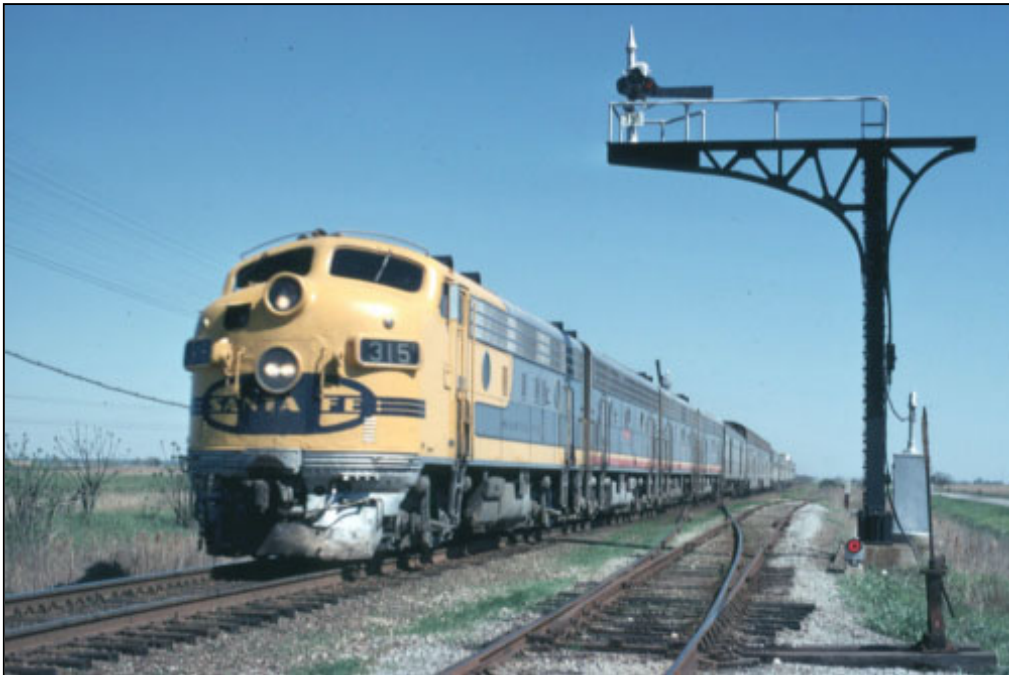
The 315L leads No. 16 past a pair of vintage semaphores at Orchard, Texas on March 17, 1973. Orchard is located at MP 76.2 on the Southern Division Third District. This was ATS territory and the maximum authorized speed for passenger trains at this location was 90 MPH. -Ralph Back
