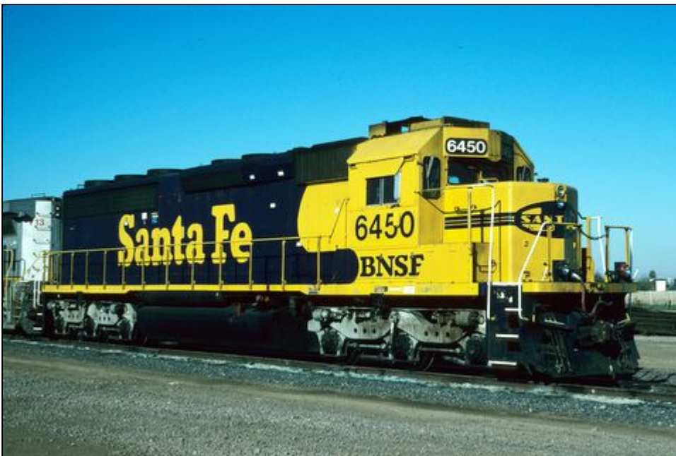
Left - BNSF SD45-2 6450, originally ATSF SD45-2 5669/SPSF SD45-2u 7200/ATSF 5800, is typical of the BNSF renumbering patch; and has white step edges and white front and rear step hand rails, a BNSF modification. Riverbank, CA 2-8-03. - Kodachrome Ralph Back collection
