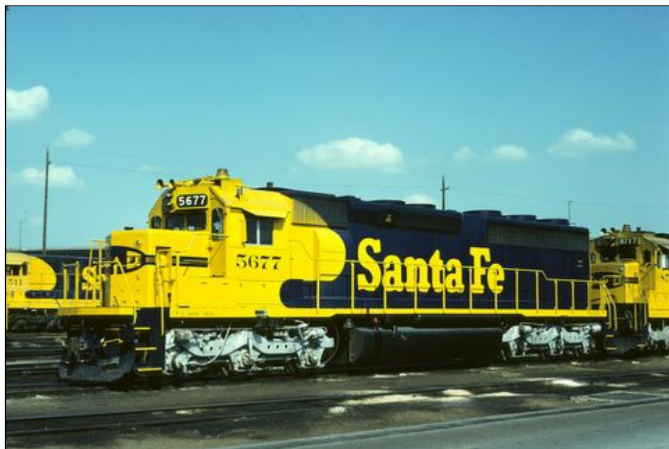
Right - ATSF SD45-2 5677 has been repainted and now has yellow step edges and yellow front anti-climber, "Santa Fe" lettering style, and silver painted trucks. The 5677 was remanufactured to SPSF SD45-2u 7208 in March 1986 and later renumbered 5808, and is on the BNSF roster as BNSF 6458. Kansas City, KS 9-4-78. - Kodachrome Ralph Back collection
