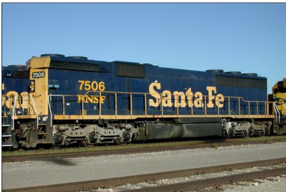
Left - BNSF SD45-2B 7506, originally ATSF SD45-2 5703/SD45-2B 5512, is typical of the BNSF SD45-2B renumbering patch. BNSF 7506 is shown in the surge fleet storage line, and is one of the last four SD45-2Bs still on the BNSF roster but now numbered 6522. Northtown, MN 8-22-02. - Photo by Eric Goodman
