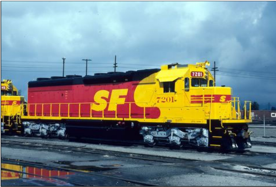
Left - Just released from remanufacturing, SPSF SD45-2u 7201 was remanufactured from SD45-2 5681 from the second order, and now has Sinclair radio antenna, and no nose classification lights. SPSF 7201 was renumbered to ATSF 5801 and was on the BNSF roster as BNSF 6451 until retired in December 2002 and sold to NRE. San Bernardino, CA 2-15-86. - Kodachrome Ralph Back collection
