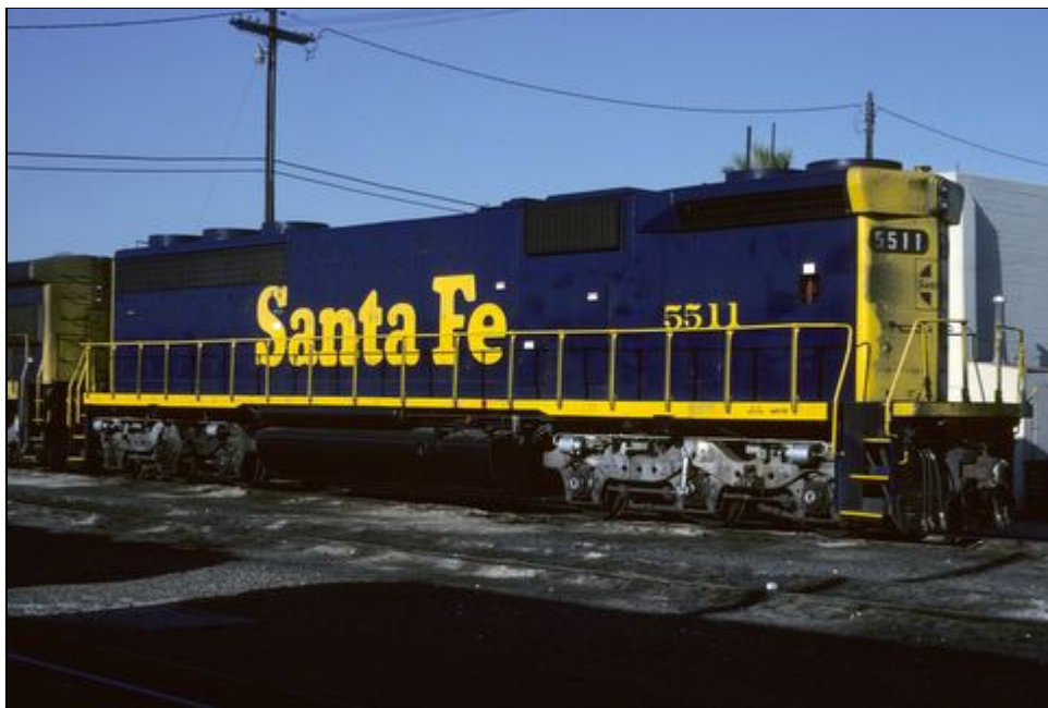
Right - ATSF SD45-2B 5511, originally SD45-2 5676, was the first SD45-2B remanufactured with the dynamic brakes on the front of the unit where the cab used to be, and has the yellow Santa Fe cross herald on the designated front. The 5511 was on the BNSF roster as BNSF 7505 until renumbered 6521 in November 2006. Phoenix, AZ 5-12-88. - Kodachrome Ralph Back collection
