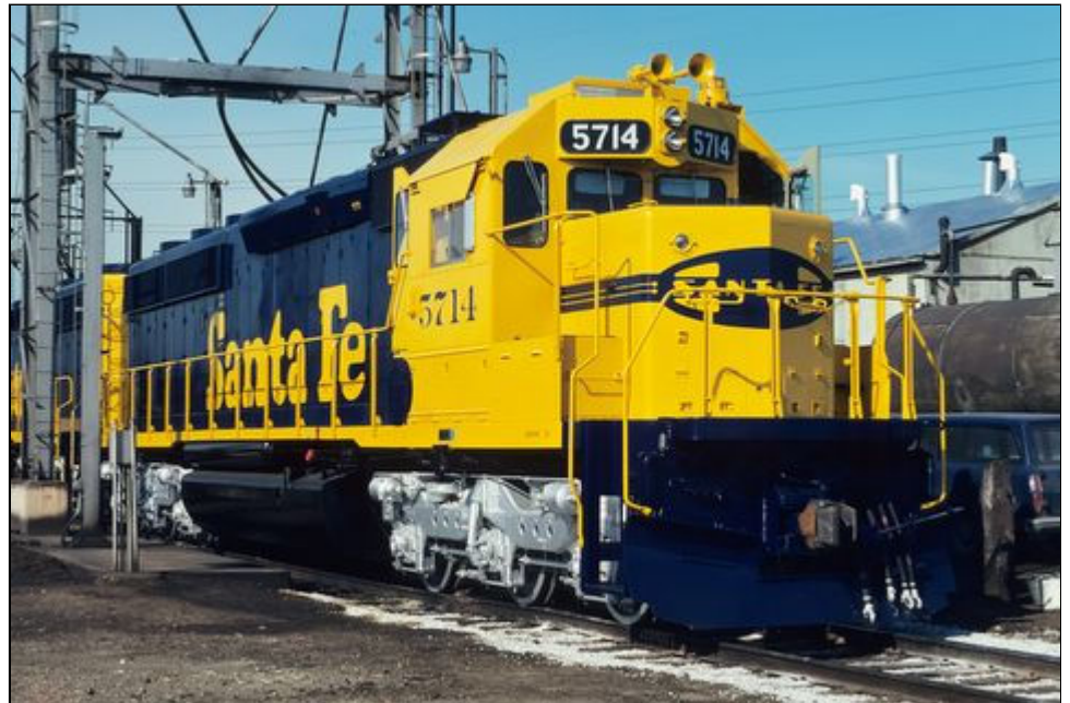
Right - ATSF SD45-2 5714 has just been delivered to the Santa Fe at Corwith Yard. The 5714 has the medium-width anticlimber with coupler lift bars with loop and silver painted trucks, and was the last SD45-2 of the third order which were leased and not owned by the Santa Fe. The 5714 has the new-style fabricated radiator intake grilles which became standard on the EMD 'Dash 2' models. Chicago, IL 6-1-74. - Joe McMillan, Ralph Back collection
