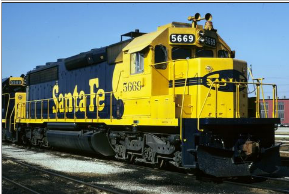
Left - ATSF SD45-2 5669 is three months old displaying its as delivered appearance in the blue/yellow Warbonnet scheme. The 5669 was the first SD45-2 remanufactured in February 1986 to SPSF SD45-2u 7200 and later renumbered 5800. You can see the small air vent mounted vertically on cab side below the front of cab window on engineer's side which caused the unit number to be noticeably off center. ATSF 5800 is on the BNSF roster as BNSF 6450. Corwith - Chicago, IL 9-1-73. - Joe McMillan, Ralph Back collection
