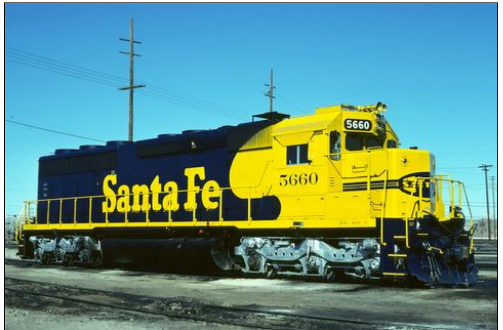
Right - ATSF SD45-2 5660 has been repainted from its as delivered blue/yellow stripe scheme to the blue/yellow Warbonnet scheme with "Santa Fe" lettering style, yellow step edges, and now has a Sinclair radio antenna and coupler lift bars with loop. The 5660 was one of the six units from the first order delivered with A/C. Note the louvers on the front cab wall below the window. The 5660 was remanufactured to SPSF SD45-2u 7204 in March 1986 and later renumbered 5804, and was on the BNSF roster as BNSF 6454 until retired in July 2002. Barstow, CA 2-20-78. - Kodachrome Ralph Back collection
